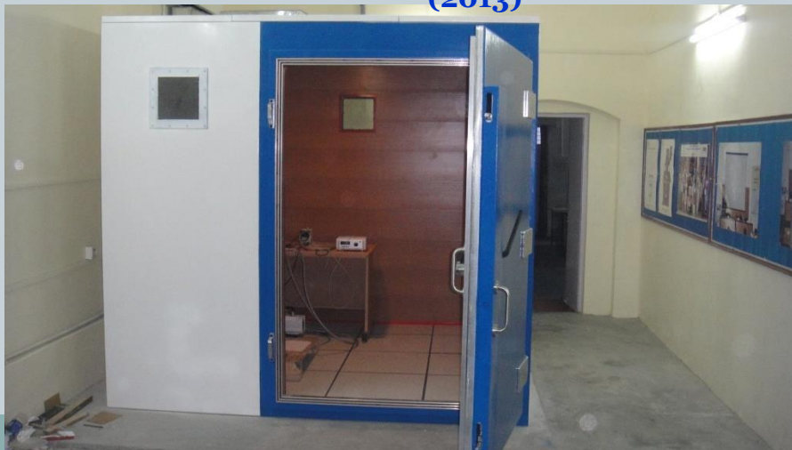
Magnetically Shielded Room
